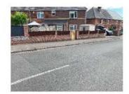
No official dropped kerb at Windsor Road – on West side, except for private drive, though this does not have any infill and is difficult for wheelchairs to traverse, risking damage to wheelchairs.
