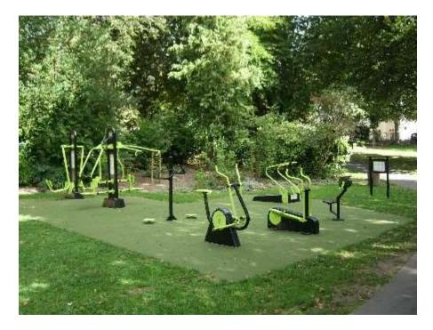
The gym site comprises the following equipment placed within a Notts Sward safety surfaced area. Whilst critical fall heights are very low (less than 800 mm) the safety surface helps to prevent erosion of the former grass surface and does provide some softening of any accidental fall. It is comprised of the following equipment: -
