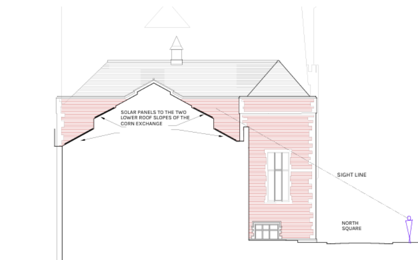
SECTION, NORTH ELEVATION
