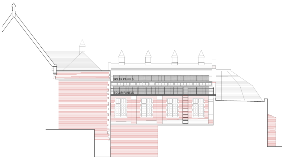
PROPOSED EAST ELEVATION WITH SOLAR PANELS
